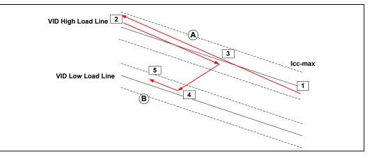
Figure 2-6 is an example of dynamic VID. The diagram assumes steady state, constant current during the dynamic VID transition for ease of illustration; actual processor behavior allows for any dIcc/dt during the transitions, depending on the code it is executing at that time. Note that during dynamic VID, the processor will not output VID codes that would disable the voltage regulator output voltage.
